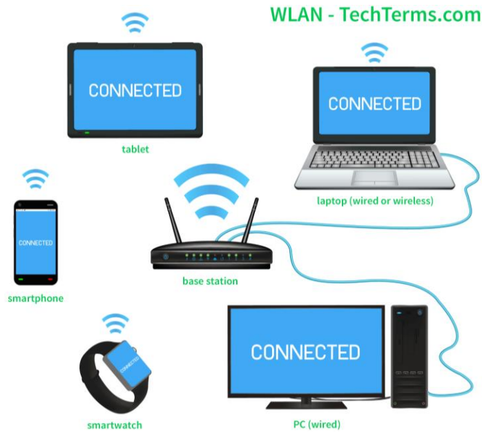
A diagram showing devices connected wirelessly in a WLAN.
