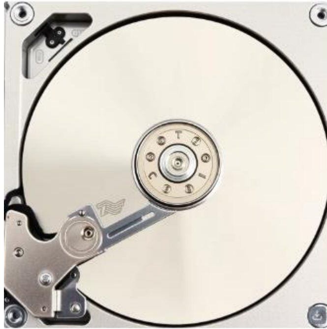
An image showing the internal components of a hard disk drive, including platters and read/write heads.
